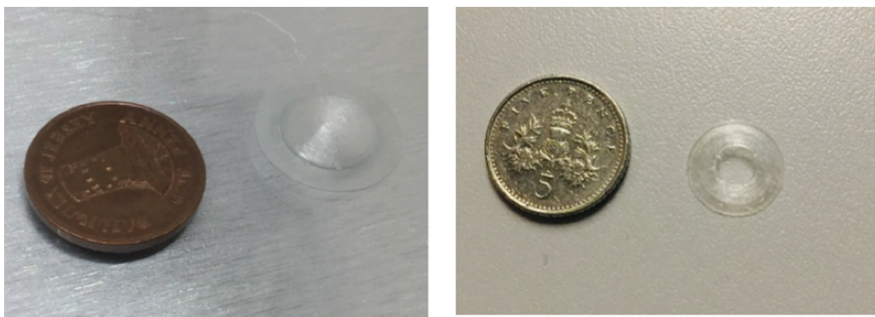
Figure 7 Blank 3D printed contact lenses with and without central aperture (5 mm) comprising of EVA/PLA 90 : 10 (wt/wt) blend.
