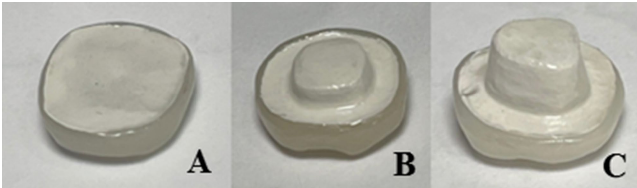
Fig. 5 Cemented composite veneers over PEEK cores A ) 0 mm depth b ) 2 mm depth c ) 4 mm depth
