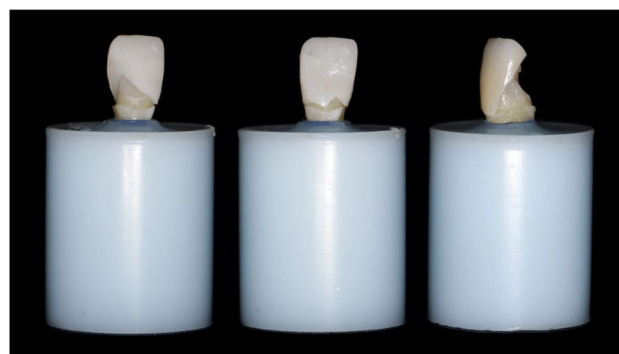
Fig. 8 Representative Type I failure pattern after fracture resistance testing
