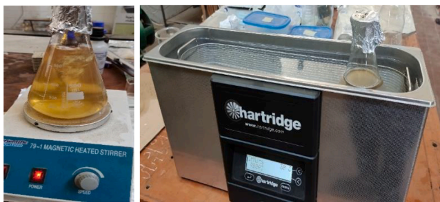
Fig. 2. Fuel preparation stages. a) Stirrer setup; b) Sonicator setup.
