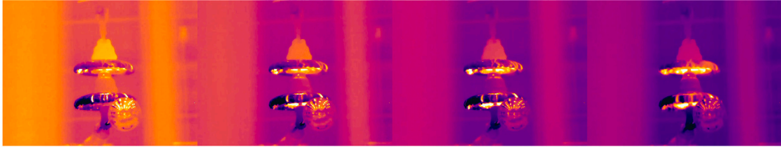
Fig. 2. Progressive frames from the dataset depicting Class 1: Dry band arcing only (no flashover) and Class 2: Dry band arcing leading to flashover (flashover).
