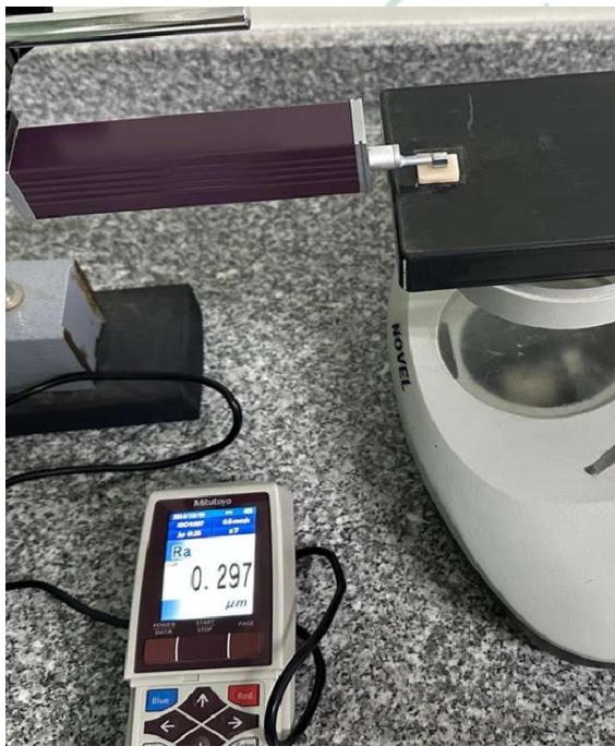
Figure 1: surface roughness testing
