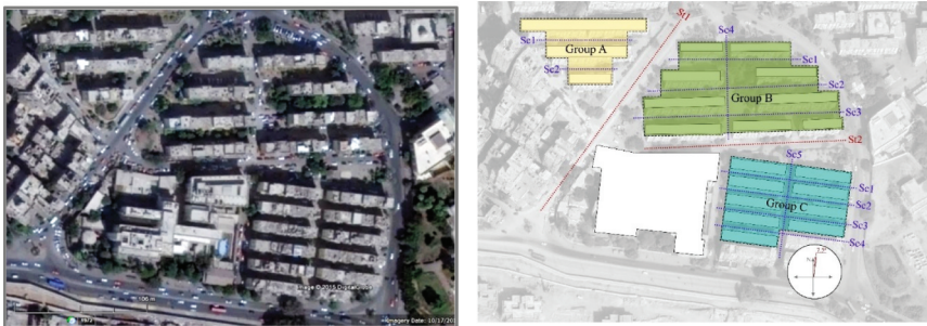
Figure 1. Linear-parallel layouts of Nasser's popular housing (1956–1970). Left, Zeinhom area of study (google earth pro 7.3, coord. 30.021519569282766, 31.24426831474131); right, streets and block types.
