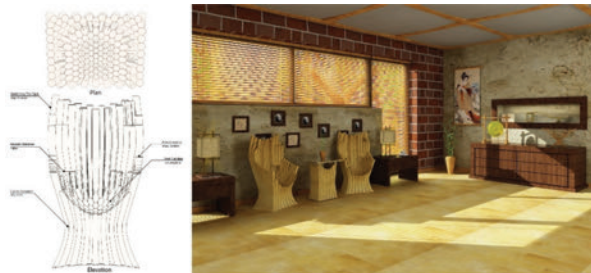
Figure 11. The orthogonal projection of the fabricated chair (Left). Final render after editing on 3Ds Max (Right).
