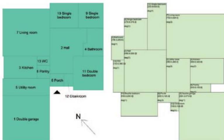
Fig. 19 An example of the generated floor plans using Nisztuk & Myszkowski ‘s method [24]
