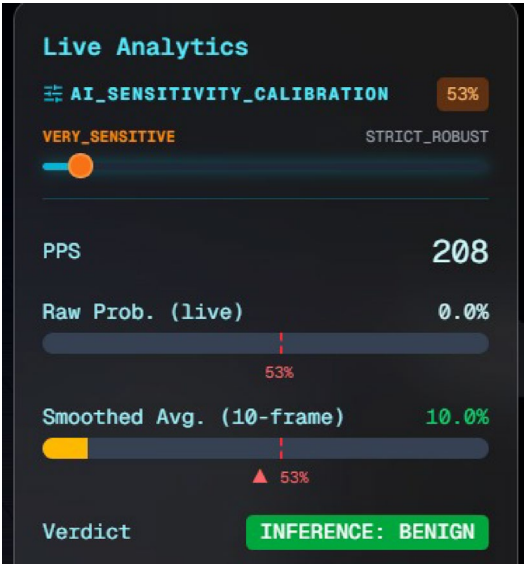
Fig. 10. The Live Analytics interface of the FedShield-IDS dashboard, showcasing the real-time AI Sensitivity Calibration slider set at 53%. The panel tracks active Packets Per Second (PPS), raw instantaneous threat probability (0.0%), and the 10-frame smoothed rolling average (10.0%), outputting a stable benign evaluation verdict.
