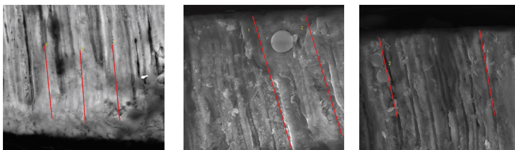
Figure-6 Image analysis representing the degree of penetration of a) Varnish, b) p(NIPAM) and c) Mix on superficial dentin using ESEM with magnification 1500 x after immediate testing.
