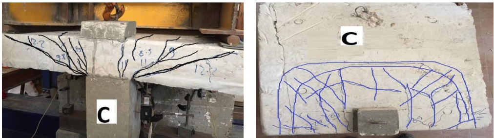
Fig. 30. Cracking pattern for specimen (C).
