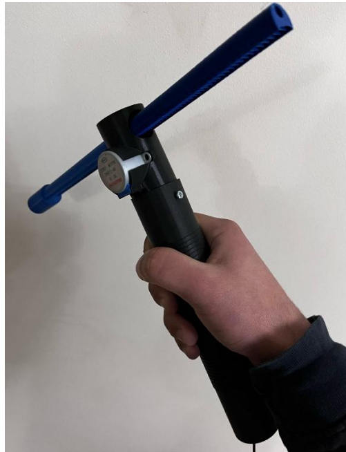
Figure 4. Electrode Holder Implementation
