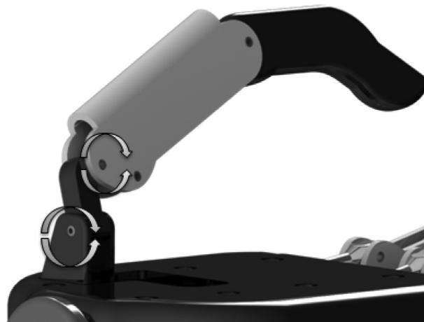
Fig. 2. The thumb architecture.
