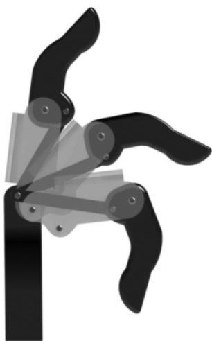
Fig. 1. Architecture for the four fingers.
