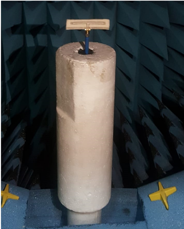
Fig. 4 The setup for measuring the standalone inspired FDA radiation pattern.
