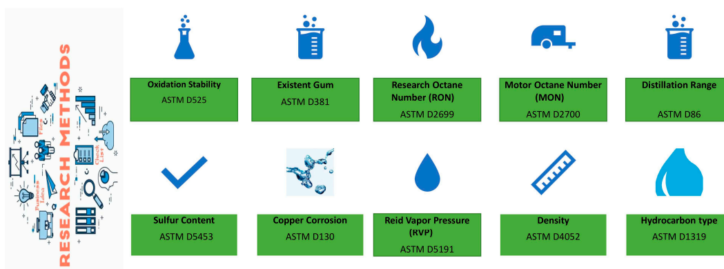
Figure 5. Research the ASTM test method for measuring the physical and chemical properties of gasoline.
