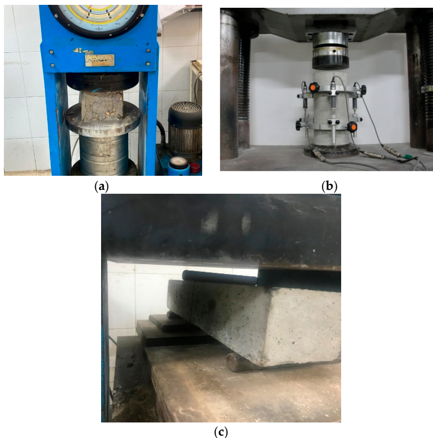
Figure 2. Test setup for all concrete specimens. (a) Compression test. (b) Young's modulus test. (c) Flexural strength test.
