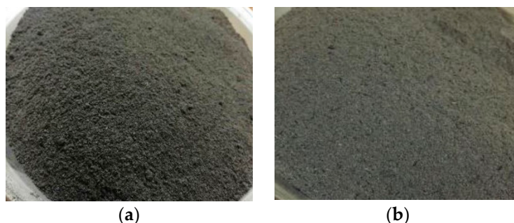
Figure 1. The shape of raw and processed SCBA. (a)—Raw SCBA. (b)—Processed SCBA.
