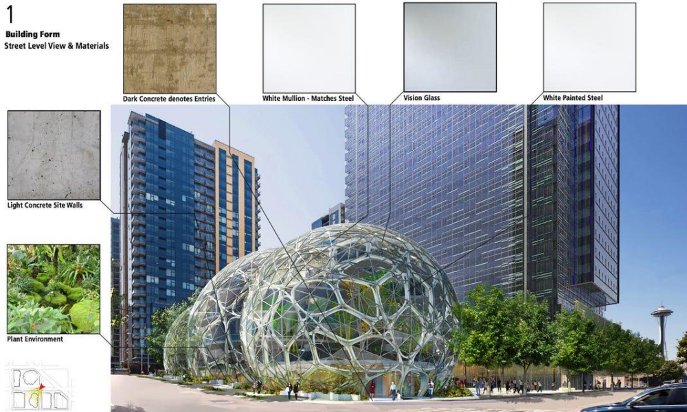
fig. 22 Materials of the sphere [37]
