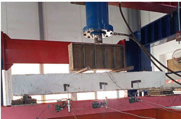
FIGURE 5 Test setup for all concrete beams.
