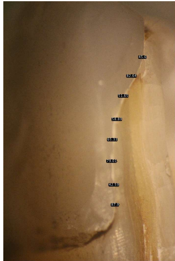
Figure 5. Measurement of the incisal external margin adaptation after thermocycling of e.max sample using image j software.
