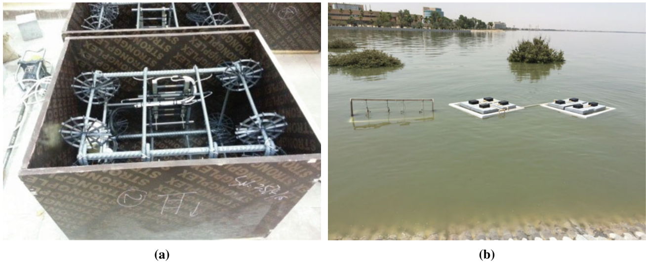
Fig. 2 Installation and setting up of corrosion sensors (a). Concrete specimens with embedded sensors under testing in the tidal zone (b)
