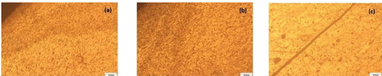
Fig. 10 Microstructure of (T6) heat treatment at 1500 rpm, dwell time 8 s
