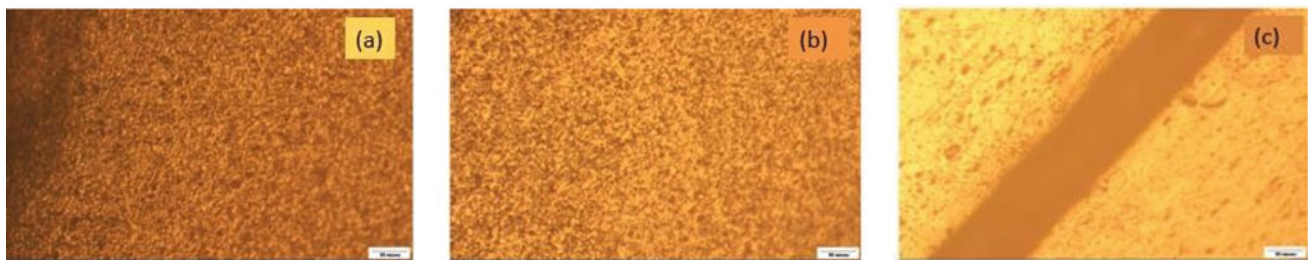
Fig. 9 Microstructure of (O) heat treatment at 1500 rpm, dwell time 8 s
