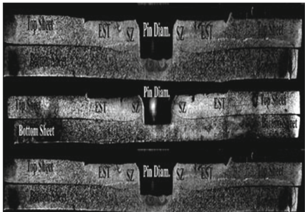
Fig. 7 Macrostructure of (T6) heat treatment of the welded joints at 1500 rpm and dwell time values (6, 8 and 10 s)
