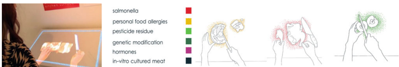
Fig. 19 Bio-Detecting Kitchen Surface detect the presence of harmful components by changing the colour of the countertop
