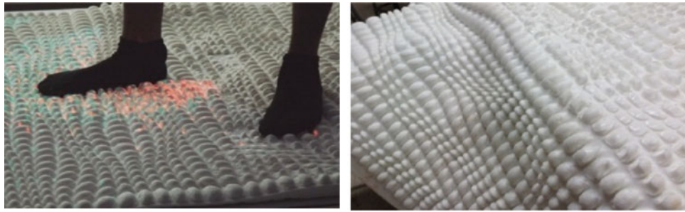
Fig. 30 The Bio detecting Floor prototype is a smart biomaterial designed by a student called Tashia Tucker in Philadelphia research, Drexel University. That Bio-detecting floor is embedded with synthetic bacteria that eat dirt and toxins to clean space users' feet (Alyn Griffiths| 13 November 2013 (2015, September 14))
