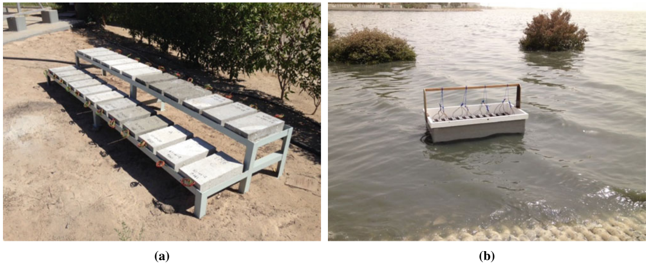
Fig. 1 Concrete specimens at the atmospheric zone (a). Concrete specimens at the tidal zone (b)
