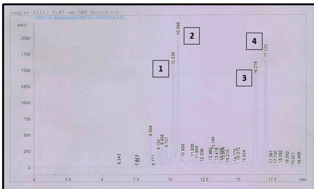
Figure 2. HPLC chromatographic profile of the bioactive ethyl acetate/ n -butanol fraction (EtFr), showing major compounds (1–4) at Rt 10.2, 10.6, 16.2 and 17.0 min, respectively.
