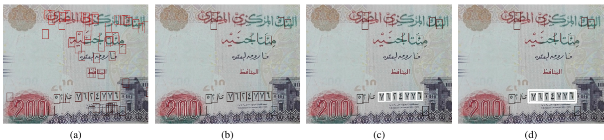
Fig. 5. Image segmentation: (a) Displaying all the borders without any filtration; (b) Filter the borders by width, height and aspect ratio; (c) Extract the digits on the serial numbers; (d) Extract the whole serial number
