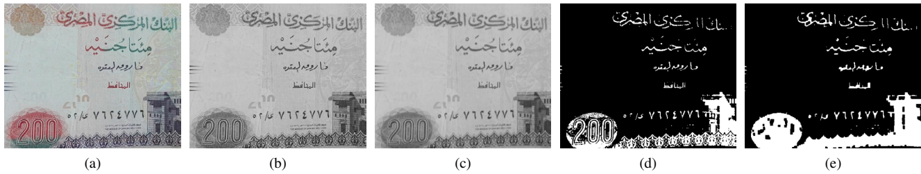
Fig. 4. (a) The original(RGB) image of 200 Egyptian pounds banknote; (b) The grayed image; (c) The blurred image; (d) Image binarization; (e) Morphological filtering
