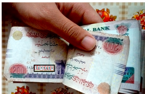
Fig. 3. Counting money using fingers scrolling and the system detects the serial number location in real-time
