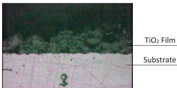
Fig. 73.6 Optical micrograph of the deposited Titania film on the condition of 40 mm as deposition distance
