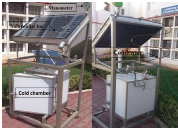
Fig. 78.3 Photograph and plan of adsorptive solar refrigerator [19]
