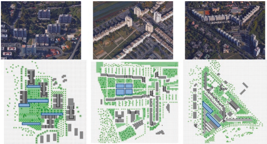
Fig. 22.1 Aerial views of the social housing districts selected as case studies and model plans of the proposed scenarios with urban design strategies for UHI mitigations: left, Pineto; middle, Torrevecchia; right Vigne Nuove
