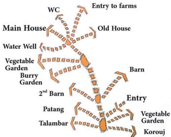
Fig. 7.5 Access to the main building and service buildings in site plan (Taleghani 2011a, b)
