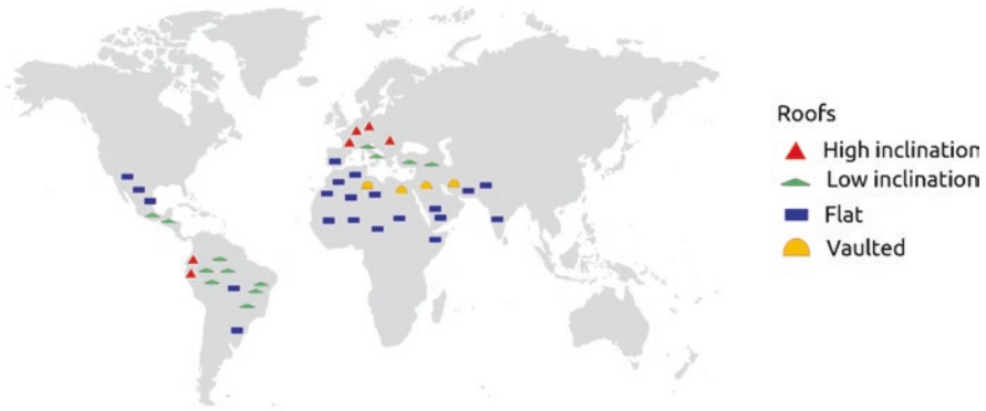
Fig. 13.1 Vernacular architecture. A map developed by Victor Olgay in Design with Climate stresses the connection between construction systems in vernacular architectures and climatic conditions throughout the world (image elaborated starting from data reported in “ Design with Climate ”)
