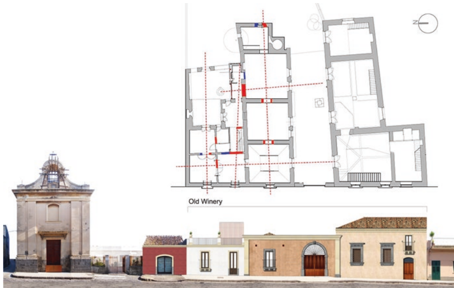
Fig. 13.7 Plan and facade of the winery in Aci Platani. Red lines on the plan show alignment of doors and windows in order to facilitate view, daylight distribution and air across the plan
