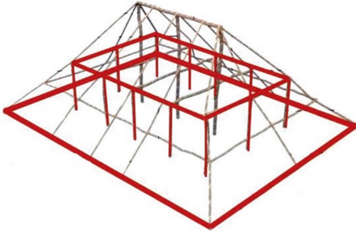
Fig. 7.22 Pitched roof structural elements (Taleghani 2010a)
