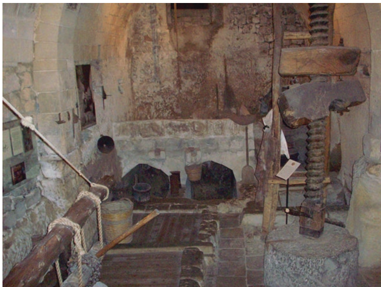
Fig. 13.6 The interior of a winery in Sicily with the torchio holding the mill stone on the right side
