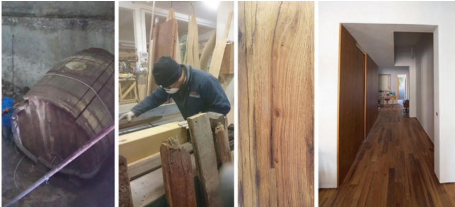
Fig. 13.11 Five barrels of 5000 L and 2.4 m diameter have been disassembled in order to provide materials enough for producing the wooden floor. Elements have been cut in a way to minimize waste
