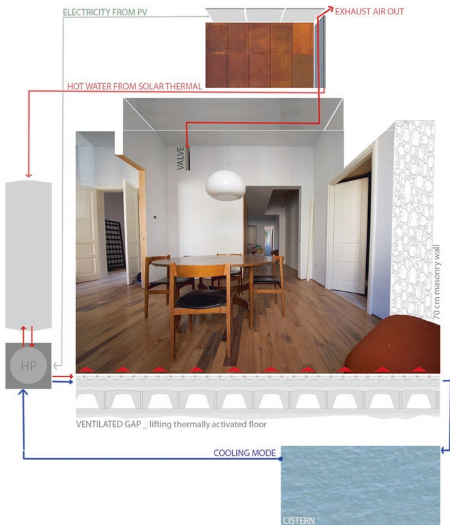
Fig. 13.9 A section of the building showing the integrated systems for enhancing the environmental performance of the existing structure. Wooden surface of the floor has been obtained cutting wood obtained by disassembling chestnut barrels
