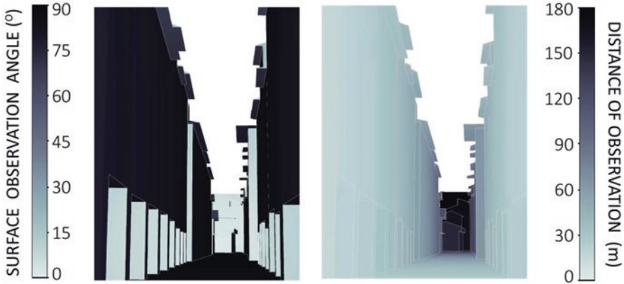
Fig. 9.6 Angle and distance of observation between the IR camera and the target calculated over a 3D model of the Rue des Tonneliers from a perspective point of view
