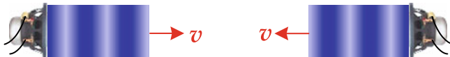
Fig. 16.5 Two identical sound sources emitting traveling waves towards each other, each with a speed v . When the two waves overlap, they produce standing waves (not shown in the figure)
