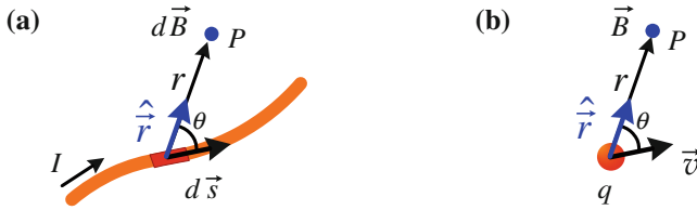
Fig. 26.1 (a) The differential magnetic field vector d\vec{B} at point P , which is located by a position vector \vec{r} drawn from a differential current element I d\vec{s} to P . (b) In case of a point charge q moving with a velocity \vec{v} , the magnetic field \vec{B} is related to the product q\vec{v}
