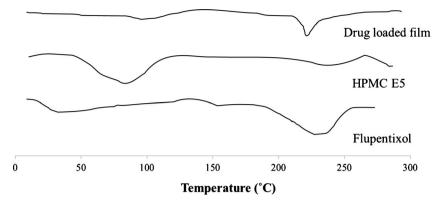
Fig. 3. Differential scanning calorimetry thermograms of flupentixol, HPMC E5, and drugloaded film
