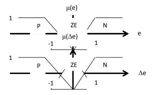
Figure 3. The Membership Function of error "e" and the error change "  $\Delta e$ "
