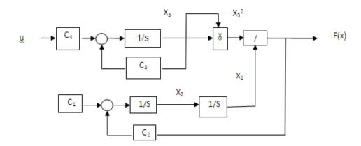
Figure 5. Block diagram of the Magnetic Ball Suspension
